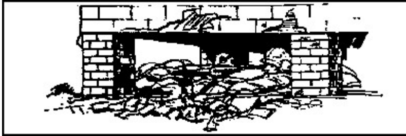
Figure 2-43. Sandbagged machine gun emplacement under a building
