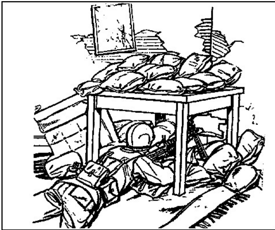
Figure 2-44. Corner machine gun bunker
